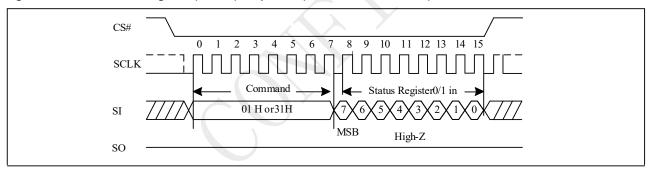
Figure 10-7a Write Status Register (WRSR) Sequence (QPI)
