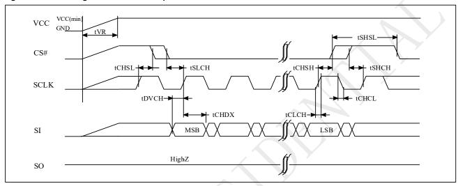
Figure 5-9 Power-up Timing
