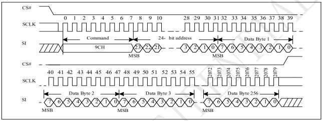
Figure 10-36a Buffer Write Sequence (QPI)
