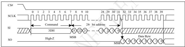
Figure 10-52a Read Block Lock Status (QPI)
