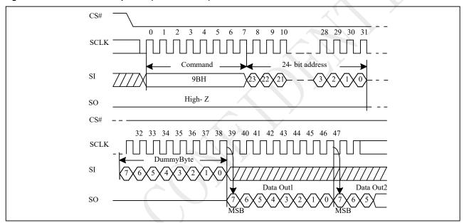
Figure 10-35a Buffer Read Sequence (QPI)
