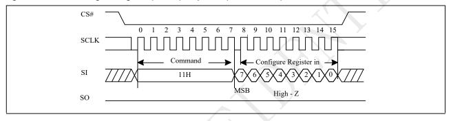
Figure 10-8a Write Configure Register (WRCR) Sequence (QPI)
