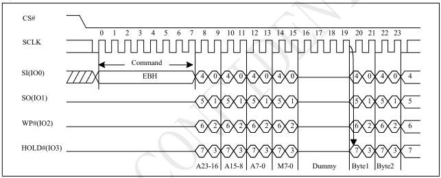
Figure 10-16 4IO Read Sequence (Command EB M5-4 ≠ (1,0))
