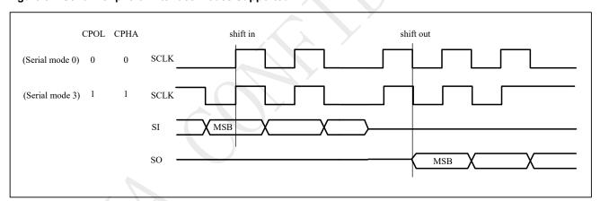
Figure 8-1 Serial Peripheral Interface Modes Supported
