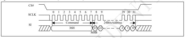
Figure 10-50a Individual Block Lock(QPI)
