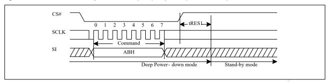
Figure 10-42c Release from Deep Power-down (RDP) Sequence (QPI)
