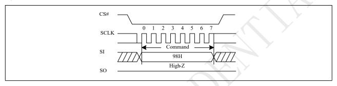
Figure 10-54a Global Block Unlock(QPI)
