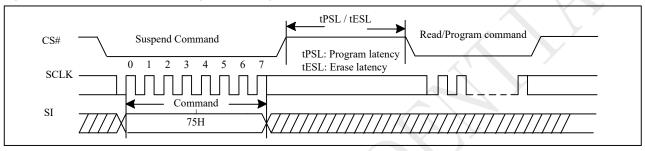
Figure 10-48a Suspend to Read/Program Latency(QPI)
