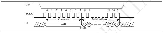
Figure 10-34a Buffer Load Sequence (QPI)
