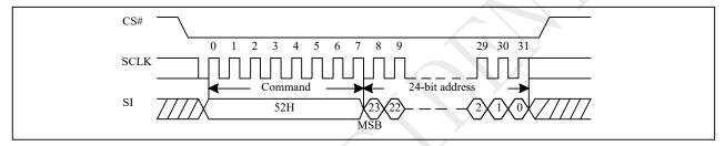
Figure 10-28a Block Erase 32K(BE32K) Sequence (QPI)
