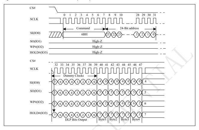
Figure 10-23c 4IO Read and Burst Read with DLP bits output Sequence
