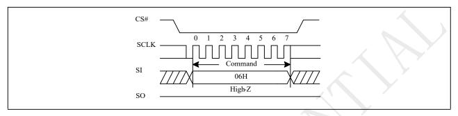
Figure 10-2a Write Enable (WREN) Sequence (QPI)
