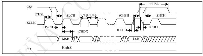
Figure 5-5 Output Timing
