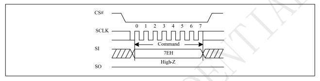
Figure 10-53a Global Block Lock(QPI)
