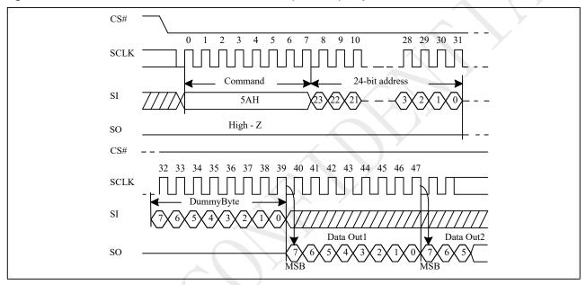
Figure 10-58a Read Serial Flash Discoverable Parameter (RDSFDP) Sequence(QPI)
