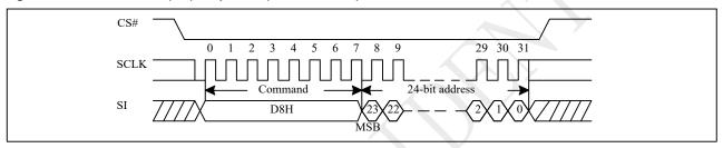
Figure 10-29a Block Erase (BE) Sequence (QPI)
